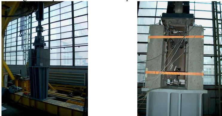
Figure 3. Testing arrangement and disposition of displacement transducers
