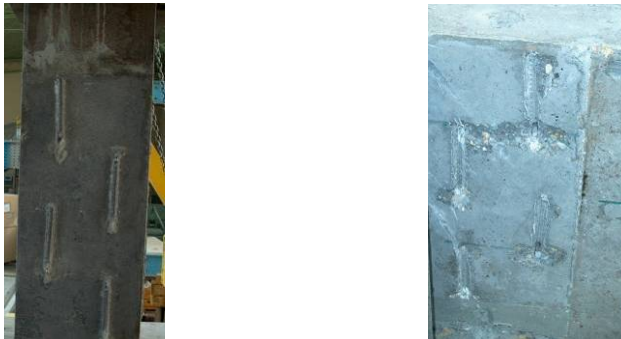
Figure 11. Shear failure type for reinforcement anchor hoops and for profiled steel plate.
