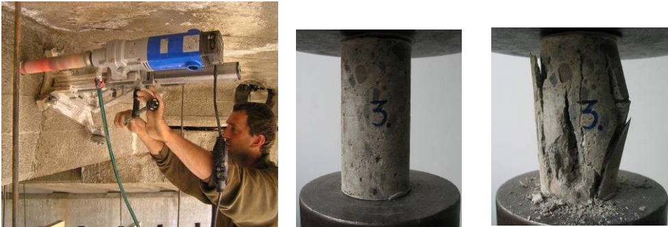
Figure 7. Extraction of samples and laboratory tests
