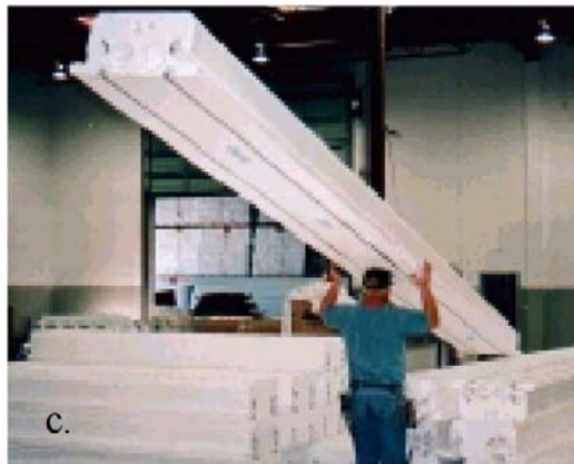
Figure 14. Insulated forming systems for floors under roof:
