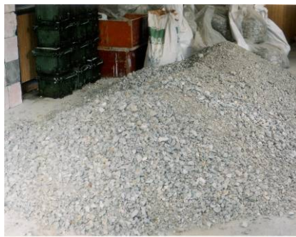
Fig. 6 – Material after secondary crushing
