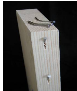
Fig. 7 Failure modes, sheathing damage and characteristic holes in timber
