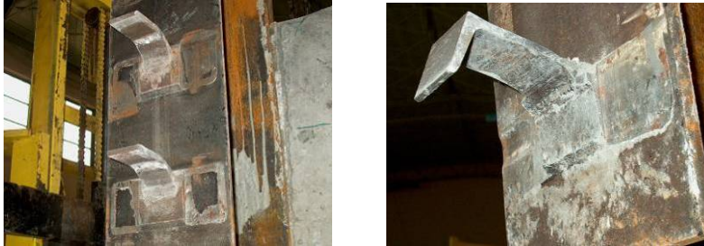
Figure 10. Shear failure for LL and UPN profiles
