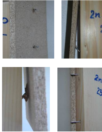
Fig. 7 Failure modes, sheathing damage and characteristic holes in timber
