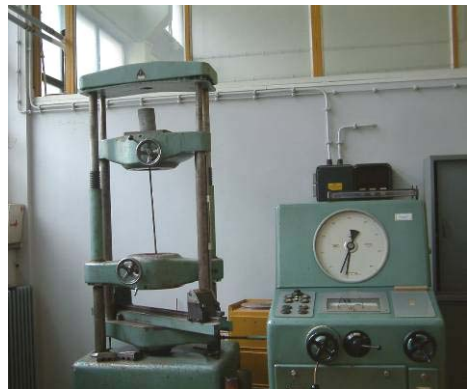
Fig. 4 – Testing of bond between concrete and reinforcement
