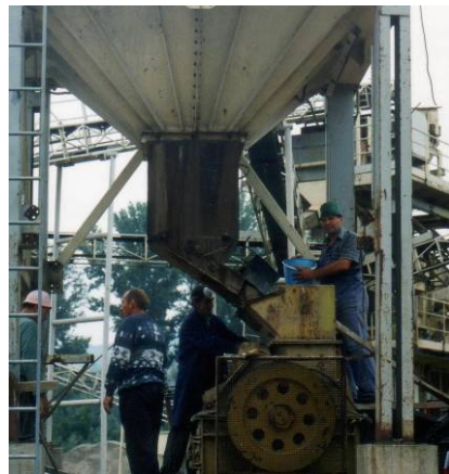
Fig. 4 – Rotation crusher
