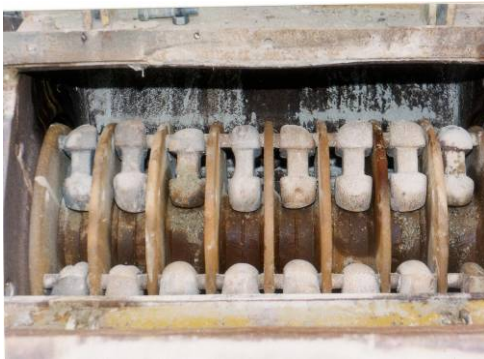
Fig. 3 - Rotation crusher (detail)
