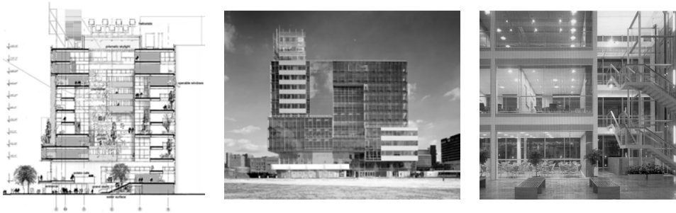
Figure 8, 9: Inner atrium for passive ventilation-section and elevation (Genzime Centre, by Behnisch, Behnisch & Partners); Figure 10: Glazed atrium as a social spot, two sided illumination of the offices obtained (John Menzies Headquarters by Bennets Associates)
