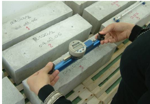
Fig. 1 – Measuring of drying shrinkage
