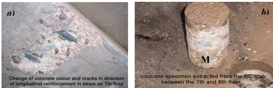
Figure 1. Change of concrete color of RC elements
