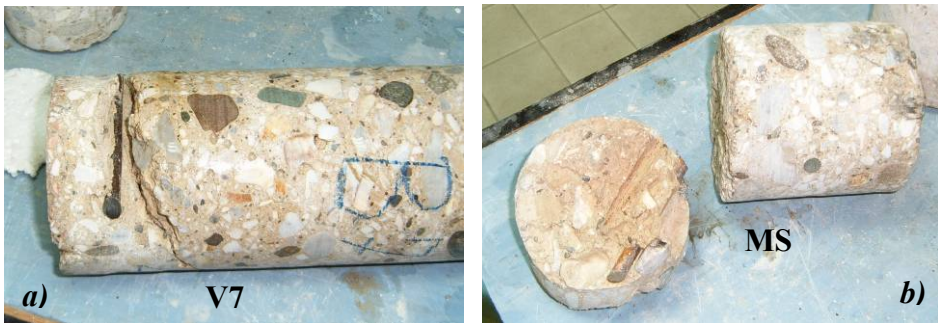
Figure 2. Change of concrete color and deterioration of surface layers of specimens
