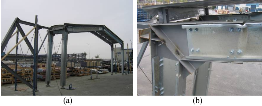
Figure 5. C1 frame: global view (a) and local buckling of the left beam connection (b)
