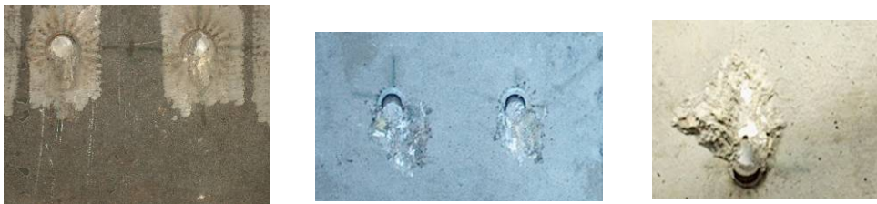
Figure 9. Typical shear failure for headed studs.
