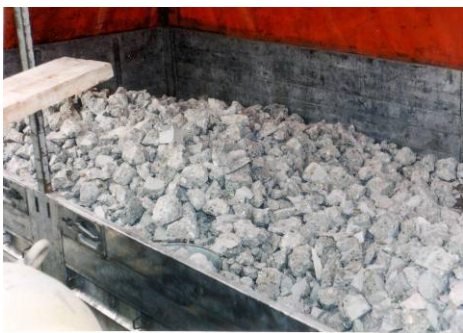
Fig. 5 – Material after primary crushing
