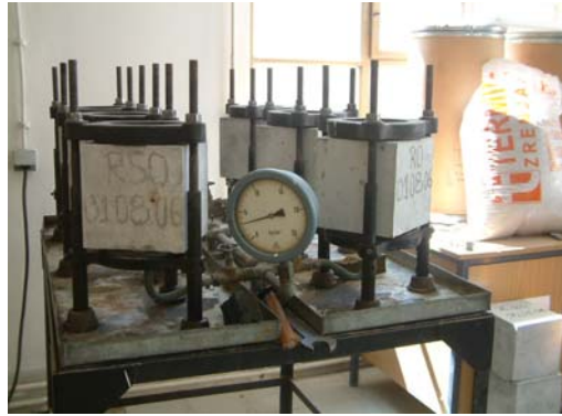
Fig. 2 – Testing of waterproofness of concrete R50
