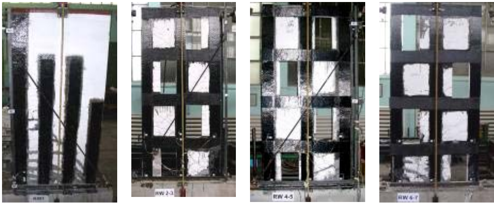
Figure 5. Reinforced concrete structural walls retrofitted and tested
