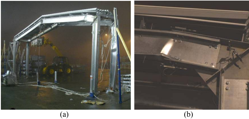
Figure 7. C2 frame: global view (a) and local buckling of the right beam connection (b)
