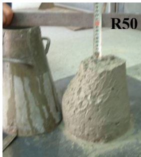
Fig. 8 – Consistency (slump test)
