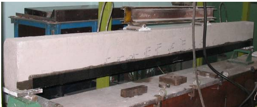
Figure 12. The consolidated beam, prior to testing
