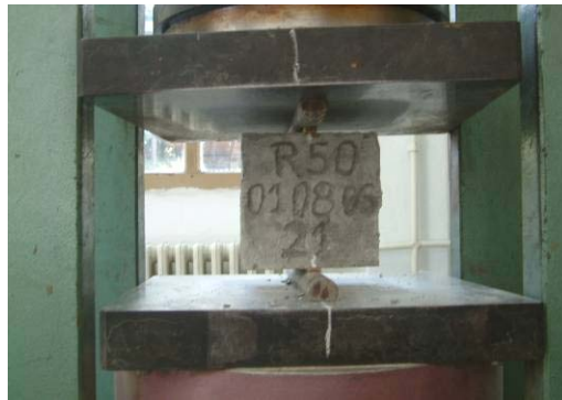
Fig. 3 – Testing of splitting strength of concrete (concrete R50)
